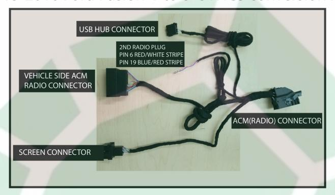
STEP 7 LOCATE THE INCLUDED CONVERSION CABLE AND PROCEED TO CONNECT IN PLACE.
