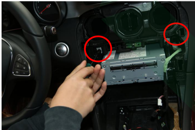
6. Remove the screws from head unit
