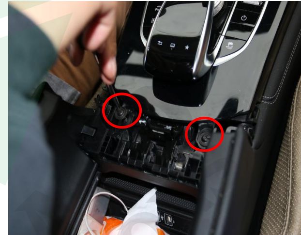
3. Remove the two screws
