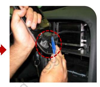
Remove the LCD case with a proper tool, be careful of the cable connected with the case.
