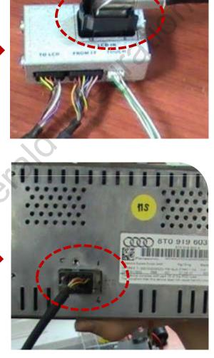
Connect the original LCD cable from monitor to "LCD-IN" of provided sub-board.
