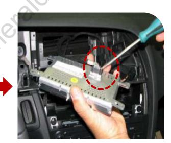
Remove the screws with a proper tool and monitor like the left picture.
