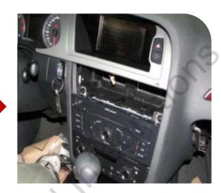
Remove the Air-Con. Box with proper tools as the left picture.
