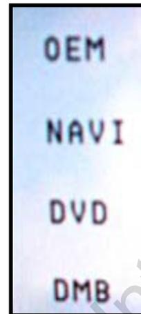
On AV2 mode, once touch the screen, Menu window appears like left picture. If no action for 5 sec or touch any other parts of the screen, this will disappear.
