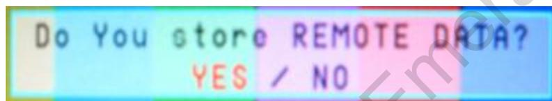
Step 5.) After all remote input finished, select "INPUT" on OSD, and press "OK" button of interface remote. Then, as left picture, confirmation window displays and ask confirmation.
