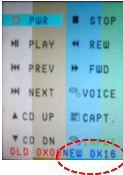
3. As soon as pressing the button, the remote button value displays at the right corner and it is saved automatically.
