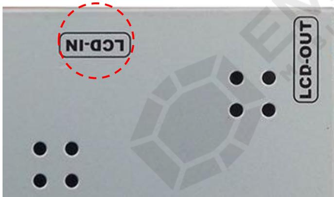
② Connect the original LCD cable with LCD-IN on the interface.
